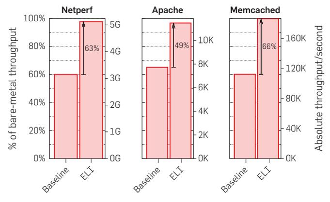
The figure shows that baseline device assignment performance is still considerably below bare-metal performance: Netperf throughput on a guest is at 60% of bare-metal throughput, Apache is at 65%, and Memcached at 60%. With ELI, Netperf achieves 98% of the bare-metal throughput, Apache 97%, and Memcached 100%. It is evident that using ELI gives a significant throughput increase, 63%, 49%, and 66% for Netperf, Apache, and Memcached, respectively.
