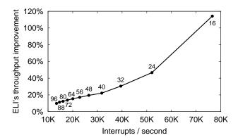
Figure 6: Throughput improvement and interrupt rate for Netperf benchmark with different interrupt coalescing intervals (shown in labels).
