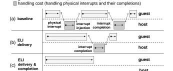
Figure 1: Exits during interrupt handling
