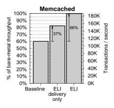
Figure 3: Performance of three I/O intensive workloads (described in the main text). We compare the throughput measured when using baseline device assignment, delivery-only ELI and full ELI, scaled so 100% means bare-metal throughput. Throughput gains over baseline device assignment are noted inside the bars.
