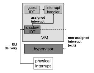
Figure 2: ELI interrupt delivery flow
